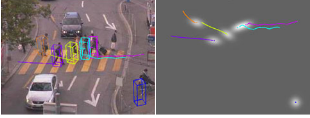
Figure 2. Influence of past trajectories on object detection. Left: 25 th frame of sequence 2, and detected pedestrians. Right: Illustration of the detection prior for the 26 th frame. Top view showing trajectories estimated in the last frame, predicted positions, and detection prior (brighter color means higher probability).
